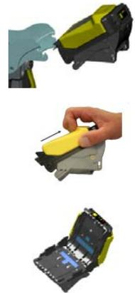
*Note: SC83 does not require the use of a cleaning card. Never use a petroleum-based product to clean this device! Petroleum based products will damage the note path. Mild non-abrasive soap is preferred over alcohol.*
