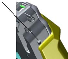
4. Once the yellow cover is released in the front, slide it back and remove it.
